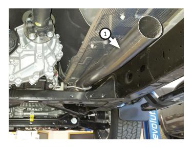
8. Place **clamp (7)** onto **intermediate pipe (2)** then connect it to inlet pipe with bend oriented upwards. Insert wire hanger into isolator and tighten clamp enough to allow for adjustment.
