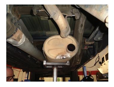
4. Apply lubricant to factory isolators (x3) shown then remove factory wire hangers (x3) from isolators. Remove trimmed factory tailpipe from vehicle.
