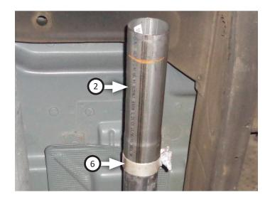
8. Place (x2) **clamps (6)** onto **muffler (3)** and connect it to inlet pipe. Tighten clamp just enough to allow for adjustment.
