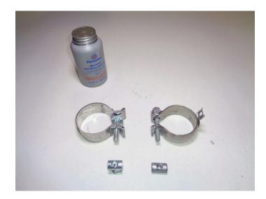
Transfer clamp from factory system onto inlet pipe
