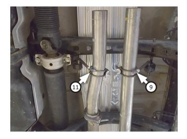
**NOTE:** If you cannot identify which muffler end connects to inlet pipes, reference drawing for proper orientation.
