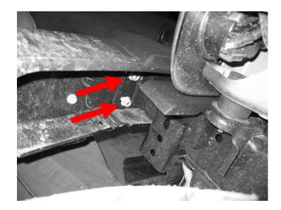
9. Using a Phillips head screwdriver, remove the four (4) screws per fog light housing that attach the fog lights to the bumper. Set the fog lights aside.
