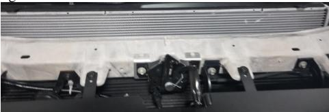
5. At this time if you have a front mount camera install in the grumper from this inside as shown. On the hold down bracket install the included foam on the camera side and trim as shown.
