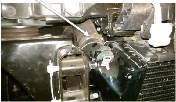
Figure 5d (PASSANGER SIDE INTERCOOLER CLAMP)
