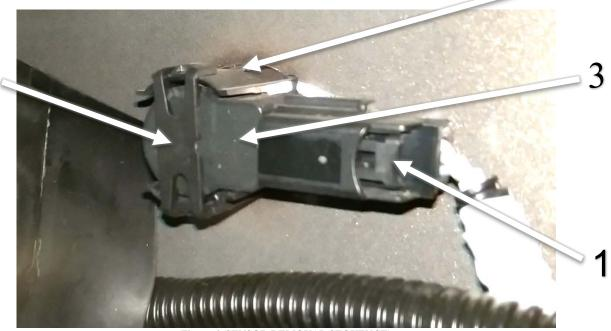
Figure 6 (SENSOR REMOVAL SEQUENCE)
