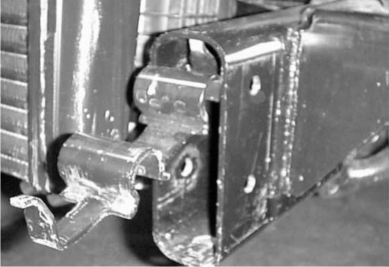
Figure 8 (FRAME ANTI-CRUSH PLATE)
