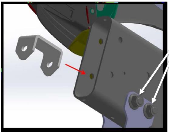
Figure 9 (FRAME ANTI-CRUSH PLATE)
