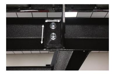
**Step 8:** After final positioning, start at the rear of the vehicle and tighten the lower portion of the bracket to 15-20 ft/lbs of torque. Continue this until all of the lower have been tighten then move to the top bolt and repeat the process.
