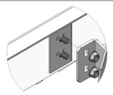
**Step 3:** Remove the factory running boards and discard.
