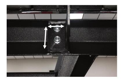
**Step. 9:** After finial positioning, completely tighten all (x6)  $\frac{1}{2}$ " -20 x  $\frac{3}{4}$ " in the pinch weld attachment.
