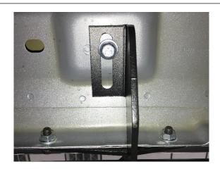
Step. 6 Next, start all (x6) 1/2-20" x 3/4" hex bolts, (x12) M8 flat washers, (x6) 5/16" lock washers and (6) ¼"-20 HC Nut in the pinch weld mounting locations and leave loose for now.
