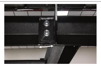
**Step 11:** Adjust the step rail to where you have approximately ¼" gap between the body of the vehicle and the top of the rail.
