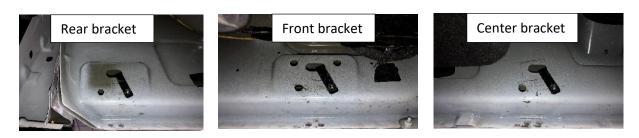
U-clip positioning. NOTE: Clips will also face forward for passenger side.
