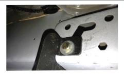
**Step 7:** Insert the black zinc M8 flanged bolts and flanged nuts in the pinch weld holes and leave loose for now.
