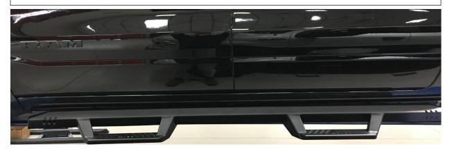
**<u>Step 12</u>**: After final adjustment, tighten all rocker panel brackets to 30 ft./lbs. **<u>Step 13</u>**: Re-peat steps 2-8 for passenger side.
