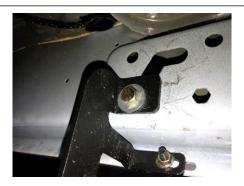
**Step 10:** Next, adjust the step assembly up/down and front/back to level out the step rail with body panel and then tighten step to brackets at 20 ft. /lbs.
