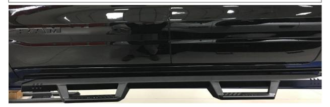
**Step 12:** After final adjustment, tighten all rocker panel brackets to 30 ft./lbs. **Step 13:** Re-peat steps 2-8 for passenger side.
