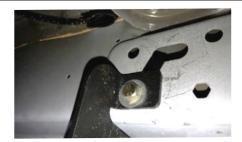
**Step 7:** Insert the black zinc M8 flanged bolts and flanged nuts in the pinch weld holes and leave loose for now.
