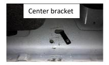
U-clip positioning. NOTE: Clips will also face forward for passenger side.
