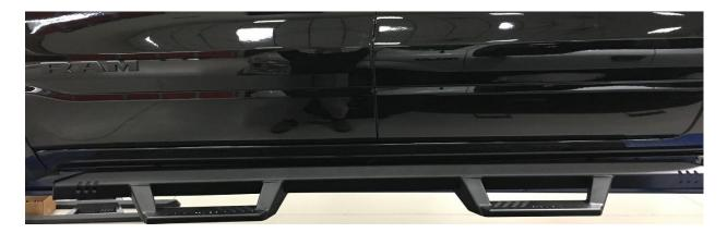
**<u>Step 8</u>**: After finial adjustment, tighten all rocker panel brackets to 30 ft./lbs.
