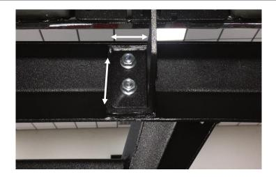
**<u>Step 7</u>**: Adjust the step rail to where you have approximately <sup>1</sup>/<sub>4</sub>" gap between the body of the vehicle and the top of the rail.
