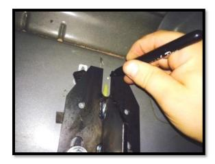
**Step 7:** Remove Nerf Step and set aside. Next, slide the additional 3/8 threaded clip from the upper rectangle hole and align with the "U" shaped mark. Make a mark through the threaded part of the clip.
