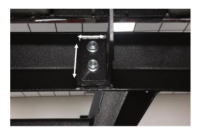
**Step 7:** After final positioning, start at the rear of the vehicle and tighten the lower portion of the bracket to 15-20 ft/lbs of torque. Continue this until all of the lower have been tighten then move to the top bolt and repeat the process.
