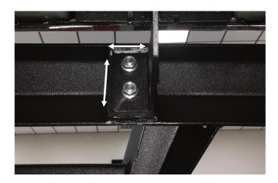
**Step 7:** After final positioning, begin at the rear bracket and tighten the lower bolt to 15-20 ft. /lb. Continue to the front bracket and then to the center bracket. Next, tighten the upper mounts from front to back at 15-20 ft. /lb.
