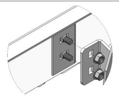
**Step 3**: Look on the underside of the body and locate the factory supplied mounting positions. **NOTE**: Some vehicles require the use of speed clips and nuts, which are supplied with the hardware kit.
