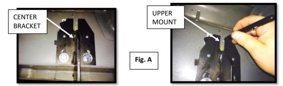
**<u>Step 8:</u>** Remove Nerf Step and set aside. Next, slide the 3/8 threaded clip from the upper rectangle hole and align with the "U" shaped mark from step 5. Make a mark through the threaded part of the clip. *Fig B*
