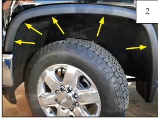
Remove (5) factory installed screws.
