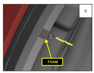
Install (7) MT1-0034 foam tabs around the stock fender trim where the grease pencil marks were made.
