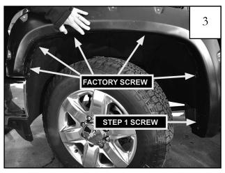
Install front flare using (5) factory screws and the (1) screw removed in Step 1.
