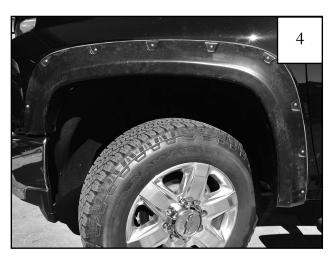
Completed front flare installation. Repeat procedure for opposite side.
