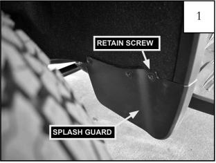
Remove the front splash guard using a T-15 Torx driver and retain (1) screw for later use.
