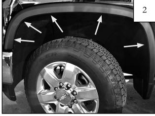
Remove (5) factory installed screws.
