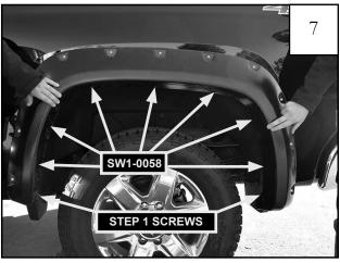
Install rear flare using (7) SW1-0058 truss screws and the (2) outboard screws removed in Step 1.
