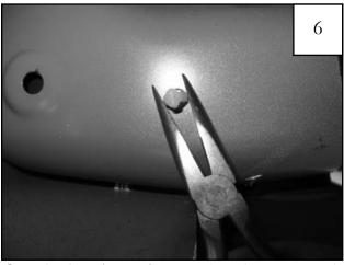
Once the three factory fasteners have been removed, reach in behind deflector to find white factory retainer. Using pliers, pinch retainer and push towards wheel center, releasing deflector. Discard factory fasteners and deflector.
