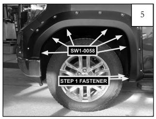
Install front flare using (6) SW1-0058 truss screws and the (2) screws removed in Step 1.
