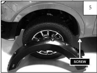
Remove (1) factory installed screw from the rear of the fender trim using a T-25 Torx driver.
