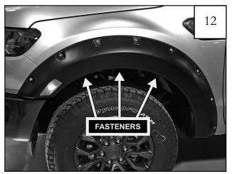
Reconnect the turn signal wiring connector and set the flare in place. Hold flare to vehicle and install (3) 1/4" panel retainers (RV1-P008) into the wheel well holes indicated. Press firmly on the flare while installing fasteners.
