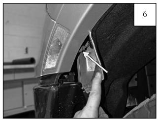
Pull back the fender liner near the front of the fender and locate the turn signal assembly and wiring.
