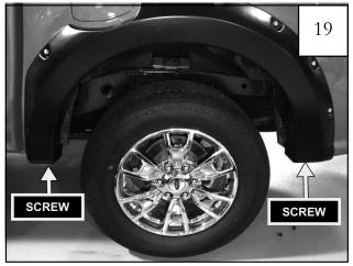
Reinstall (2) T-25 Torx screws previously removed from rear flare in Step 17.
