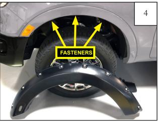
Remove (3) factory installed plastic fasteners from the driver side front wheel well using a phillips screwdriver. Needle nose pliers may be needed to extract the fasteners.
