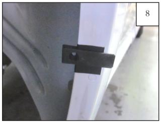
Install a Clip (CL1-0009) over each of the four Tabs (MT1-0034) placed over the upper 4 marks made in Step 6.
