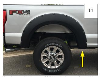
Start a supplied screw (SW1-0050) through the flare into the clip installed in Step 9. Tighten all screws.
