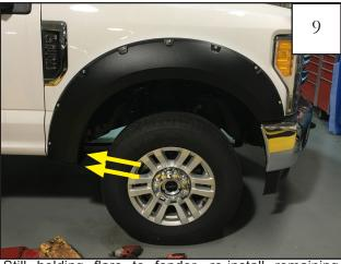
Still holding flare to fender, re-install remaining factory screws removed in Step 4 using 7mm socket and wrench. Tighten all screws.
