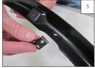
Attach 3 "U"clips (CL1-0028) to the inner bracket as shown.
