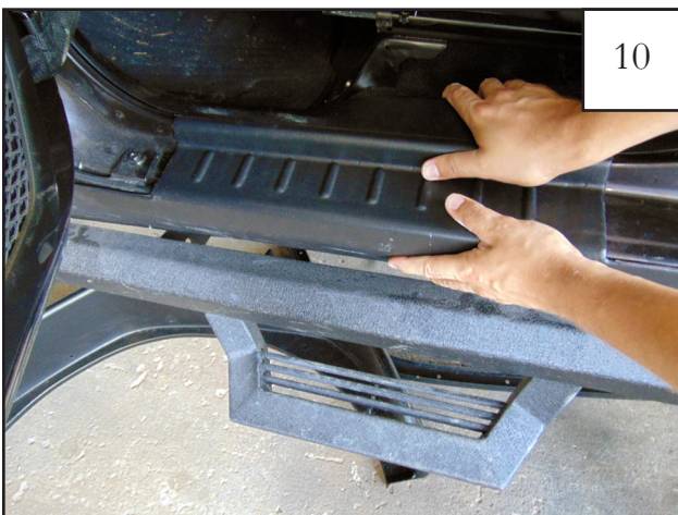
Once all tape liners are peeled, press down on entire length of part applying strong force to taped areas. NOTE: The tape reaches maximum adhesive bond after 24 hours of contact. Do not wash vehicle for 24 hours.
