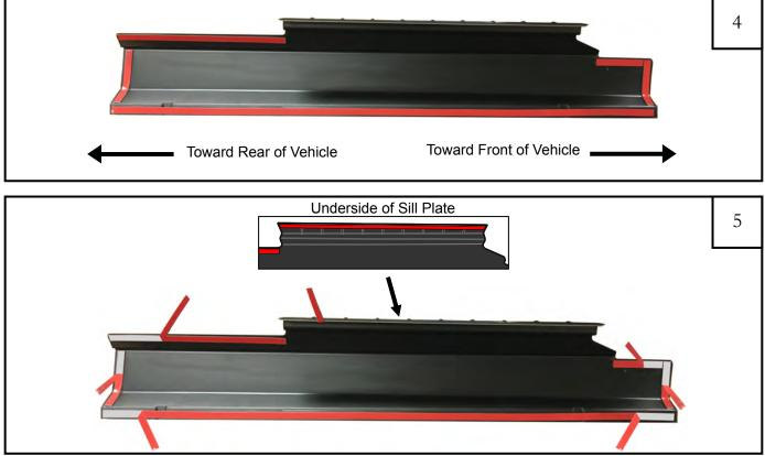
Peel back roughly 3" of red tape liner from the pieces of tape on the back side of the front part. Make sure red tape liner will be accessible when part is attached to truck.
