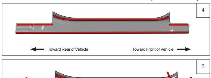
Peel back roughly 3" of red tape liner from the pieces of tape on the back side of rear part. Make sure red tape liner will be accessible when part is attached to truck.
