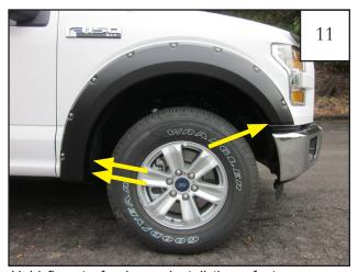
Hold flare to fender, re-install three factory screws removed in Step 4 using sockets and wrench.
