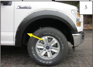
Hold flare to vehicle and mark one flare hole location with a grease pencil.
