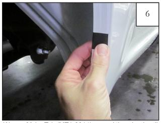
Wrap a Mylar Tab (MT1-0014) around the wheel well sheet metal, centered over each of the three marks made in Step 5.
