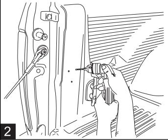
Cut out supplied template and tape to the D-pillar as shown. Using a center punch, mark holes as specified by the template.
