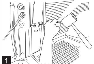
Using a power drill and 9/64" drill bit, drill through the sheet metal. If equipped with a bedliner, drill through bedliner.
