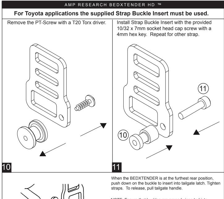
NOTE: Ensure that buckles are properly inserted into latches by pulling on the straps after both buckles have been inserted.
