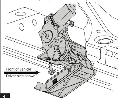
Install motor linkage B in the the First mount position at the front of the truck on the Driver side, using the bolts supplied (12). All plastic or rubber hole plugs need to be removed that are next to the linkage mounts. Torque fasteners to 16 ft-lbs. (22 N m).
