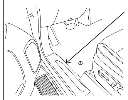
Remove the driver side door sill trim and and kick panel carefully. Pull up the carpet, and poke a small screwdriver through the rubber insulation material.
