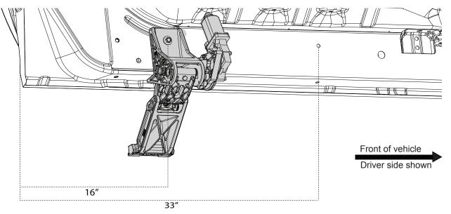
Assemble the motor to the linkage like the picture before installation shown on page 2. **Position the motor so the linkage is in the mid extension position.** This way the lower bolt can still be installed.
