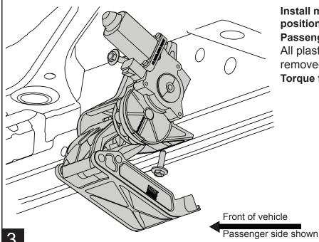
Install motor linkage A in the the First mount position at the front of the truck on the Passenger side, using the bolts supplied (12). All plastic or rubber hole plugs need to be removed that are next to the linkage mounts. Torque fasteners to 16 ft-lbs. (22 N m).
