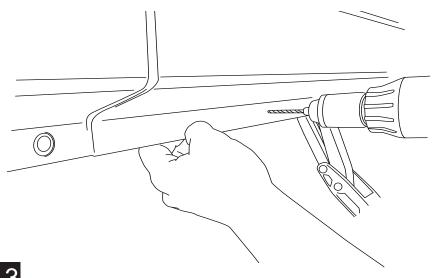
Center punch and drill a 1/8" pilot hole then drill a 19/64" hole through the pinch weld at marked locations. Deburr all holes. After drilling apply paint to holes to prevent rusting.
