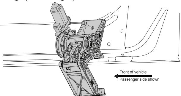
Assemble the motor to the linkage like the picture before installation. **Position the motor so the linkage is in the mid extension position.** This way the lower bolt can still be installed.
