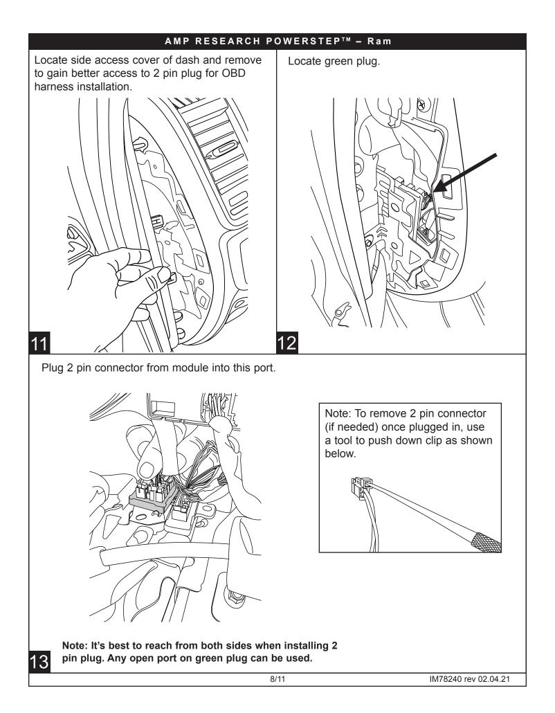
**OBD II install:** Use Supplied Posi Lock connectors to attach the Plug and Play Module to the Harness. Attach matching colors on the harness to the wires on the module. Plug in module to OBD II port on the vehicle. Secure harness with supplied tie wraps.
