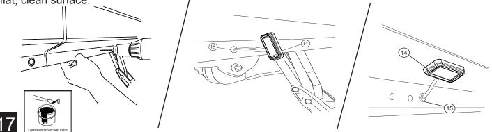
Using supplied butt connectors (13) connect the lamp wires. Red to Red, Black to Black. Once Crimped use heat gun to shrink tube. Close and wrap conduit with electrical tape. Secure all loose wires with cable ties. Pull lamp wires upward to avoid any wire snagging.
