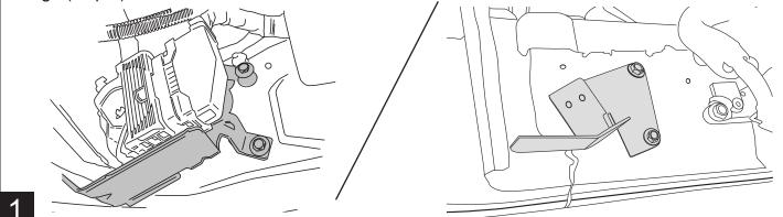
Locate mounting points. First and last set of studs on the inner sill. Motor linkage mounts towards the front of the truck and Idler towards the rear. Driver side shown below. Note: Studs may have excess paint buildup. We recommend using a wire wheel or thread repairing
