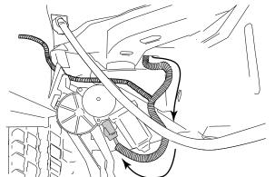
On Passenger Side, run Wire Harness leg down and along underside of the vehicle floor and frame to front Drive Linkage. Connect harness to motor and secure harness with tie wraps. Route remainder of wire harness towards rear linkage assembly for LED lights
