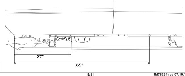
Drill a 9/32" hole through the pinch weld at marked locations. Deburr all holes.
