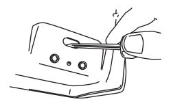
**Linkage Installation:** On rear linkages thread front hex bolt into rivet nut with washer. Note on Front drive linkages both hex bolts can be threaded into position.
