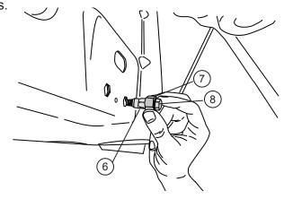
With Rivet Nut Tool held in place with 19mm wrench, tighten Hex Bolt until Rivet Nut deforms and secures itself to the sheet metal (110 in-Lbs. or 4 turns). Remove Hex Bolt and Rivet Nut Tool. Repeat for each of the four mentioned mounting locations.
