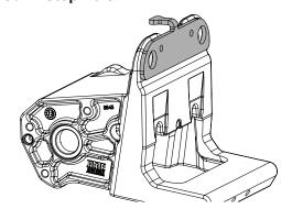
**All Linkages:** Slide linkage over pre threaded bolts. Using a T27 Torx driver start torx bolts and washers. Snug bolts but do not tighten. Replace bolts from step 15 if present.
