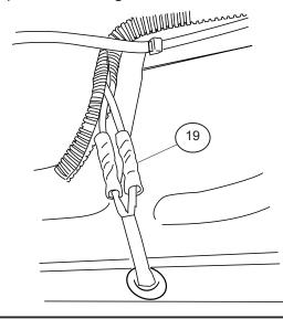
Close and wrap with conduit and electrical tape. Secure all loose wires with cable ties, with lamp wires pulled upward to avoid any wire snagging.
