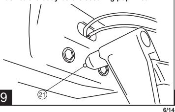
Assemble Hex Bolt (lubricated with soapy water), Washer, Rivet Tool, and Rivet Nut together as shown and place into hex cutouts in sill. An extra Hex Bolt and M8 Washer is supplied to install rivet nuts.
