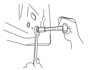
**WARNING:** Rivet Nuts not properly collapsed will not hold securely to sheet metal.
