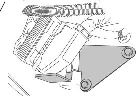
While holding brake cable adjustment nut with wrench (located on driverside along frame, towards the rear), loosen brake cable to allow for slack. Mark position of nut before loosening.
