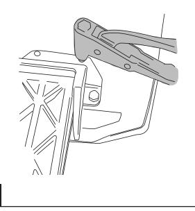
Reinstall fuse to Powerstep harness. Check that all doors activate the Power Step and the LED Lights work when doors open and close. Reinstall any remaining trim panels.
