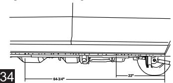
Drill a 9/32" hole through the pinch weld at marked locations. Debur all holes. After drilling apply paint to holes to prevent rusting
