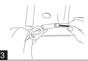
Remove brake cable guide from frame by depressing locking tabs and sliding guide out through hole. Unthread brake cable from frame mount.
