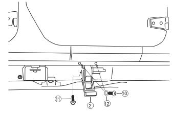
Torque fasteners to 16 ft-lbs. (22 Nm)
