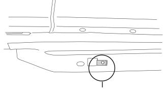
Install U nut under vehicle, middle of front door for front motor linkage as shown. (Some vehicles with factory steps may already include this u-nut)
