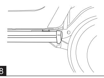
Tighten 4 socket cap screws with 3/16" allen wrench. Torque to 10 ft-lbs. (13.5 N-m)
