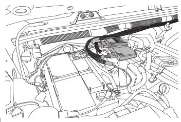
Route longest leg of wire harness across fire wall to driver side and under vehicle outside of frame rail. Route shortest leg of wire harness down fire wall and outside of frame rail on passenger side.
