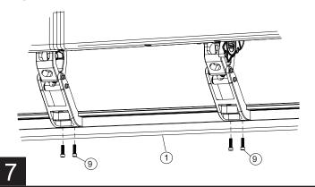
Line up rear of step extrusion with rear fender well.
