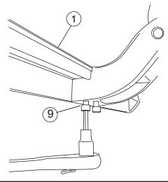
Remove fuse from Power Step wire harness.
