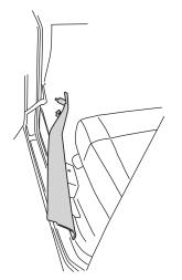
Route Violet wire under carpet to driver side door sill and connect to violet wire coming from door as shown. Note: For door removal attach posi tap on chassis side of door harness.
