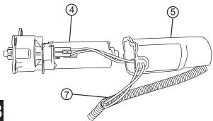
Insert plastic push pin rivets in mounting holes of motor cover. Use pliers to ease installation.
