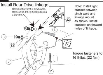
Note: Due to variances in sheetmetal, shimming may be required to allow proper retraction of steps. If needed, install shims between adaptor and upper mount.
