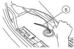
NOTE: Seal holes with silicone glue and cover with tape so carpet does not stick to glue.
