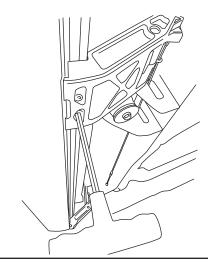
Using a 13mm socket Torque linkage bolts 4x (9) from step 4 to 16 ft-lbs Next use a 10mm socket, torque linkage spacer bolt 2x (12) from step 5 to 8 ft-lbs.
