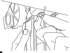
Install provided spacer (16) and M6 bolt (12) into upper mount as shown on both the Drive and Idler linkages. Do not tighten.
