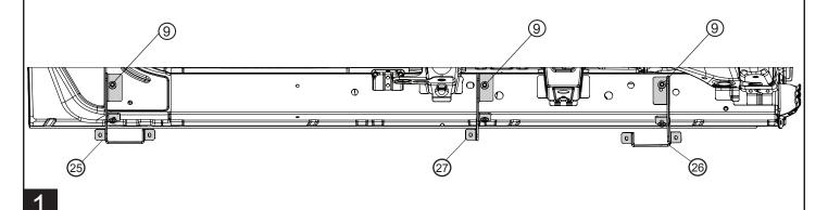
Slide 7 carriage bolts(14) into rail and position them in place to attach brackets leaving the 3rd and 5th bolt in place to use to attach Light Brackets . Use provided flange nuts (15) to attach board to brackets. Do not tighten to allow for adjustment.
