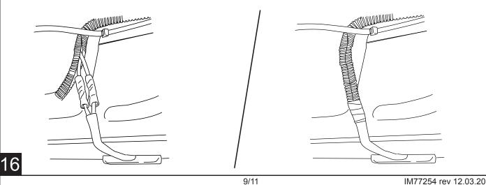
**OBD II install:** Use Supplied Posi Twist connectors to attach the Plug and Play Module to the Harness. Attach matching colors on the harness to the wires on the module. Plug in module to OBD II port on the vehicle. Secure harness with supplied tie wraps.
