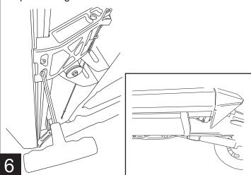
Using a 13mm socket Torque linkage bolts 4x (8) from step 5 to 16 ft-lbs Next use a 10mm socket, torque linkage spacer bolt 2x (12) from step 6 to 8 ft-lbs. Once linkages are tight cycle board to verify steps deploy under own weight.
