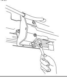
Thread supplied bolts 2x (8) into Front Drive Linkage. Repeat step for Rear Idler Linkage. Do not tighten.
