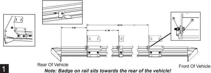
position. Starting with the rear bracket work towards the two front brackets. Slide R
