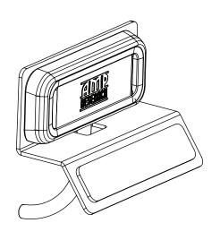
Affix LED light bracket assembly to rail. Mount front light rearward of front linkage and mount rear light just forward of rear linkage.
