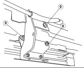
Start from rear of vehicle and Torque 5x Flange Nuts (16) to 16 ft-lbs.
