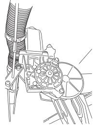
Torque bolts on mounting brackets to 16ft-lbs.
