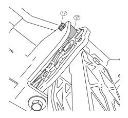
Slide mounting T-nut into position, Center board in rail pocket. Tighten fasteners to 10 ft-lbs.
