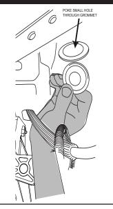
Connect harness to motor. Secure harness with tie wraps.
