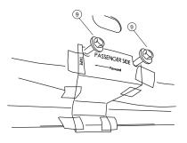
Mark appropriate holes as indicated with a center punch. Front linkage marked "Front" and Rear linkage marked "Rear".
