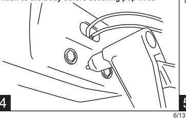
Assemble Hex Bolt (lubricated with soapy water), Washer, Rivet Tool, and Rivet Nut together as shown and place into hex cutouts in sill. An extra Hex Bolt and M8 Washer is supplied to install rivet
