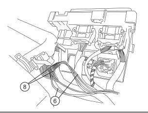
Route the two Wire Harness legs down over the wheel wells toward Motor Linkages, long leg across to the passenger side. Secure harness with tie wraps.
