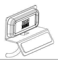
Affix LED light bracket assembly to rail. Mount front light rearward of front linkage and mount rear light just forward of rear linkage.
