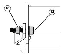
Attach motor to linkage. Using a 4mm hex Torque to 36 in-Lbs.
