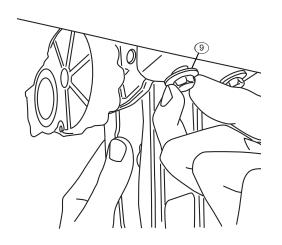
Install provided spacer (22) and M6 bolt (12) into upper mount as shown on both the Drive and Idler
