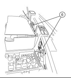
Remove fuse box lid and fuse box power lead with 13mm wrench. While depressing release tabs, lift fuse box to view bottom side.
