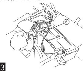
Splice Power Step trigger wires into the Door Ajar wires with provided Posi-Tap™ splicers. The Power Step trigger wires color coordinate with the factory Door Ajar wires. Follow the steps below to correctly splice wires.
