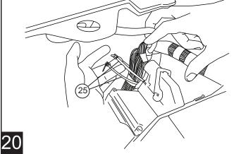
Insert controller into tie-wrap loops and cinch down securely. The tie-wraps should cinch down into channels on controller surface.
