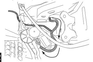
On Passenger Side, run Wire Harness leg down and along underside of the vehicle floor and frame to front Drive Linkage. Connect harness to motor and secure harness with tie wraps. Route remainder of wire harness towards rear linkage assembly for LED lights
