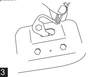
Set rivet nuts into place for alignment. Insert pop rivet through hole in plate and secure in place. Once pop rivet is installed remove string or wire from Reinforcement Plate. **NOTE: Verify plate is pulled flush to the body before securing pop rivet.**
