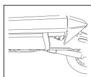
Using a 13mm socket Torque linkage bolts 4x (9) from step 14 to 16 ft-lbs. Next use a 10mm socket, torque linkage spacer bolt 2x (12) from step 15 to 8 ft-lbs. Once linkages are tight cycle board to verify steps deploy under own weight.
