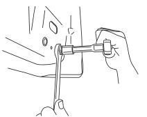
WARNING: Rivet Nuts not properly collapsed will not hold securely to sheet metal. Once rivet nuts are in place use a screwdriver to push back tab in hole to avoid interference with linkage mount.
