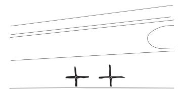
Pre drill hole using an 1/8" drill bit. Next drill holes to 9/32". Debur all surfaces. NOTE: Filing of hole may be required if drill bit wandered. After drilling apply paint to prevent rusting.
