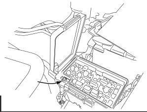
Locate and remove Black Connector with Gray latch on bottom side of fuse box (labeled "G" where connected to fuse box).
