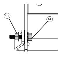
Attach motor to linkage. Using a 4mm hex Torque to 36 in-Lbs.
