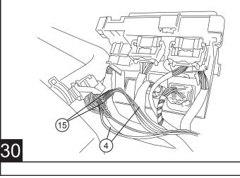
Locate and remove Black Connector with Gray latch on bottom side of fuse box (labeled "G" where connected to fuse box).
