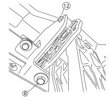
Verify rail clearance at front fender trim and push upwards on rail to ensure rail is snug to the bottom of the linkage mounting bracket. Using a 1/2" socket start at the rear of vehicle and work forward. Torque 5 flange nuts (16) to 16ft-lbs.
