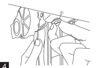
Slide mounting T-nut into position, Center board in rail pocket. Tighten fasteners to 10 ft-lbs.
