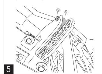
Using a 13mm socket Torque linkage bolts 4x (8) from step 5 to 16 ft-lbs Next use a 10mm socket, torque linkage spacer bolt 2x (12) from step 6 to 8 ft-lbs.
