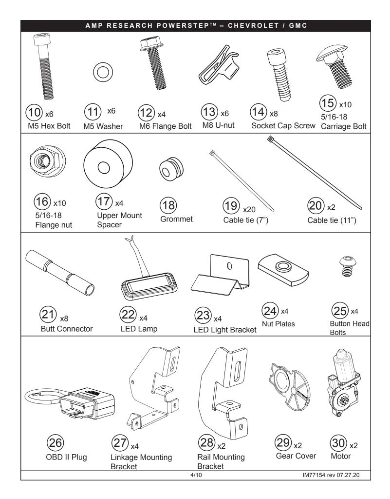
Insert and position Carriage bolts (15) into slot on rail (4). Insert from either end of rail. Using Flange Nuts (12) provided assemble Brackets 2x (27) & 1x (28) onto the rail (4). Driver side shown. Dimensions shown are for reference. Insert Threaded nut plate onto rail pocket. Light brackets will need to go rearward of Front linkage bracket and forward of Rear linkage bracket. Leave loose to allow for adjustment.
