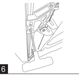
Install provided spacer (17) and M6 bolt (12) into upper mount as shown on both the Drive and Idler linkages. Do not tighten.
