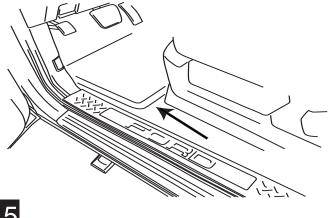
Remove grommet in floor panel above front linkage on driver side. Poke small hole into grommet and thread the two trigger wires through and up into the cabin of vehicle. Seal grommet with silicone sealer.
