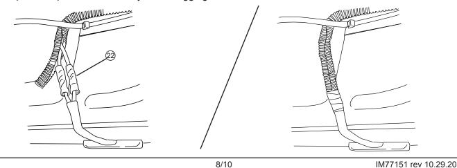
**OBD II install:** Use Supplied Posi Twist connectors to attach the Plug and Play Module to the Harness. Attach matching colors on the harness to the wires on the module. Plug in module to OBD II port on the vehicle. Secure harness with supplied tie wraps.
