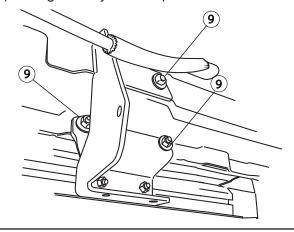
Start from rear of vehicle and Torque 5x Flange Nuts (16) to 16 ft-lbs.
