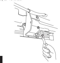
Thread supplied bolts 2x (8) into Front Drive Linkage. Repeat step for Rear Idler Linkage. Do not tighten.
