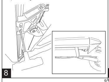
Using a 13mm socket Torque linkage bolts 4x (8) from step 5 to 16 ft-lbs. Next use a 10mm socket, torque linkage spacer bolt 2x (12) from step 6 to 8 ft-lbs. Once linkages are tight cycle board to verify steps deploy under own weight.
