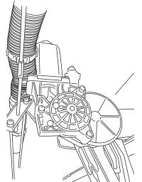
Torque bolts on mounting brackets to 16ft-lbs.
