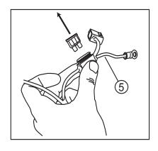
Attach wire harness to controller (make sure connector locking tabs fully engage). Mount controller with the two 11" tie wraps (#20) to factory conduit, just forward of battery.
