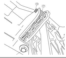
Slide mounting T-nut into position, Center board in rail pocket. Tighten fasteners to 10 ft-lbs.
