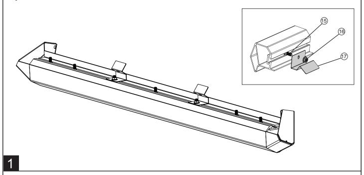
Using Flange Nuts (#16), assemble Brackets 2x (#24) & 1x (#25) onto the rail (#4), using the Carriage Bolts (#15) left from previous step (see image below for bracket placement). Next, install Flange Bolt (#13) and Flange Nut (#16) onto bracket tab. Driver side shown. Dimensions shown are for refernce.
