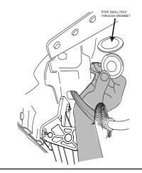
Connect harness to motor. Secure harness with tie wraps.
