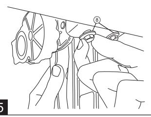
Install provided spacer (17) and M6 bolt (12) into upper mount as shown on both the Drive and Idler linkages. Do not tighten.
