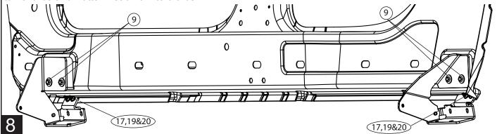
Insert and position Carriage bolts (16) into slot on rail (4). Insert from either end of rail. Using Flange Nuts (17) provided assemble rail to Brackets onto the rail. Next install Flange Bolt (14) and Flange Nut (10) onto bracket tab. Driver side shown. Dimensions shown are for reference. *Torque flange nuts to 16ft-lbs.*
