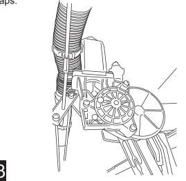
Affix LED light to bracket on rail. Mount front light rearward of front linkage and mount rear light just forward of rear linkage.
