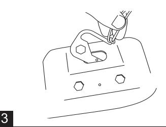
Set rivet nuts into place for alignment. Insert pop rivet through hole in plate and secure in place. Once pop rivet is installed remove string or wire from Reinforcement Plate. **NOTE: Verify plate is pulled flush to the body before securing pop rivet.**
