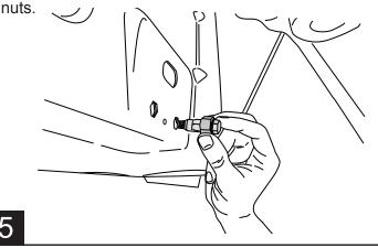
With Rivet Nut Tool held in place with 19mm wrench, tighten Hex Bolt until Rivet Nut deforms and secures itself to the sheet metal (110 in-Lbs. or 4 turns). Remove Hex Bolt and Rivet Nut Tool. Repeat for each of the four mentioned mounting locations.
