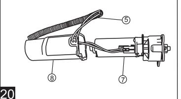
Partially separate the plastic rivet from the pin by bending the pin back and forth. Slide motor cover over motor and insert plastic push pin rivets in mounting holes of motor cover. Drive pin flush with rivet head. Use pliers to ease installation.
