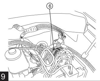
Remove power fuse. Connect wire harness to controller and secure locking clip. Connect red power lead to positive battery terminal and black ground lead to grounding lug on fender apron.
