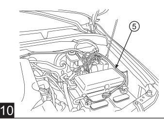
Route longest leg of wire harness across fire wall to passenger side and under vehicle outside of frame rail.
