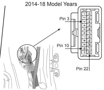
Insert plug from wire harness onto motor.
