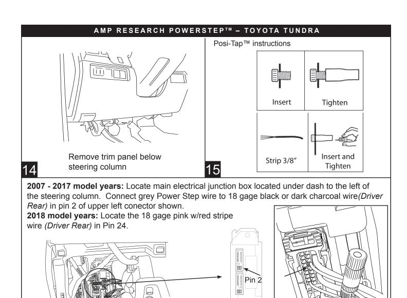
Locate 20 pin connector at bottom of panel on left. Connect blue Power Step wire to 18 gage blue wire (*Driver Front*) in pin 15 of connector shown. Plugs are located to the left of E Brake
