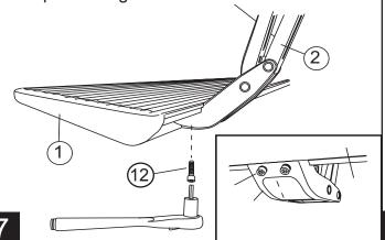
Using a 13 mm socket torque linkage bolts to 16ft-lbs. Next use a 10mm socket torque linkage spacer bolt #19 to 8 ft-lbs. Once linkages are tight cycle board to verify steps deploy under own weight and clear rail endcaps.
