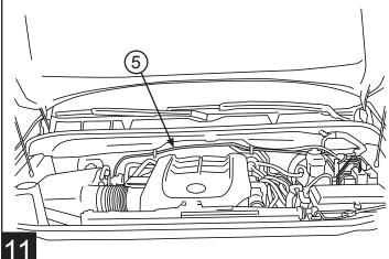
Route shorter leg of wire harness down driver side fender well and under vehicle outside of frame rail.
