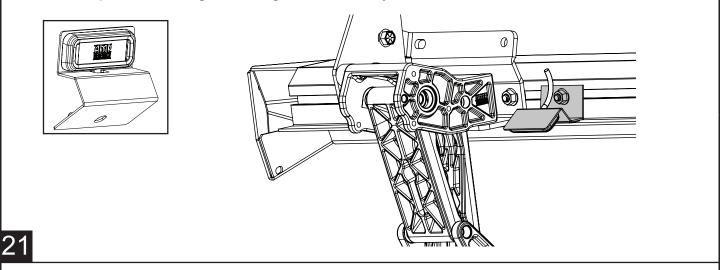
Using supplied butt connectors(22), connect the lamp wires. Red to Red, Black to Black. Once Crimped use heat gun to shrink tube. Close and wrap conduit with electrical tape. Secure all loose wires with cable ties. Pull lamp wires upward to avoid any wire snagging.
