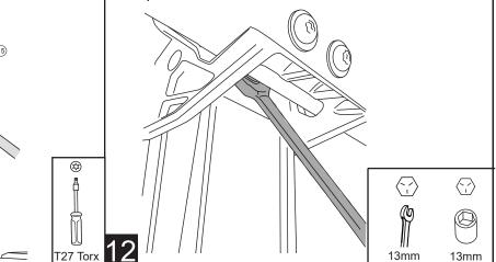
Using a T27 Torx driver torque bolts to 6 ft-lbs.
