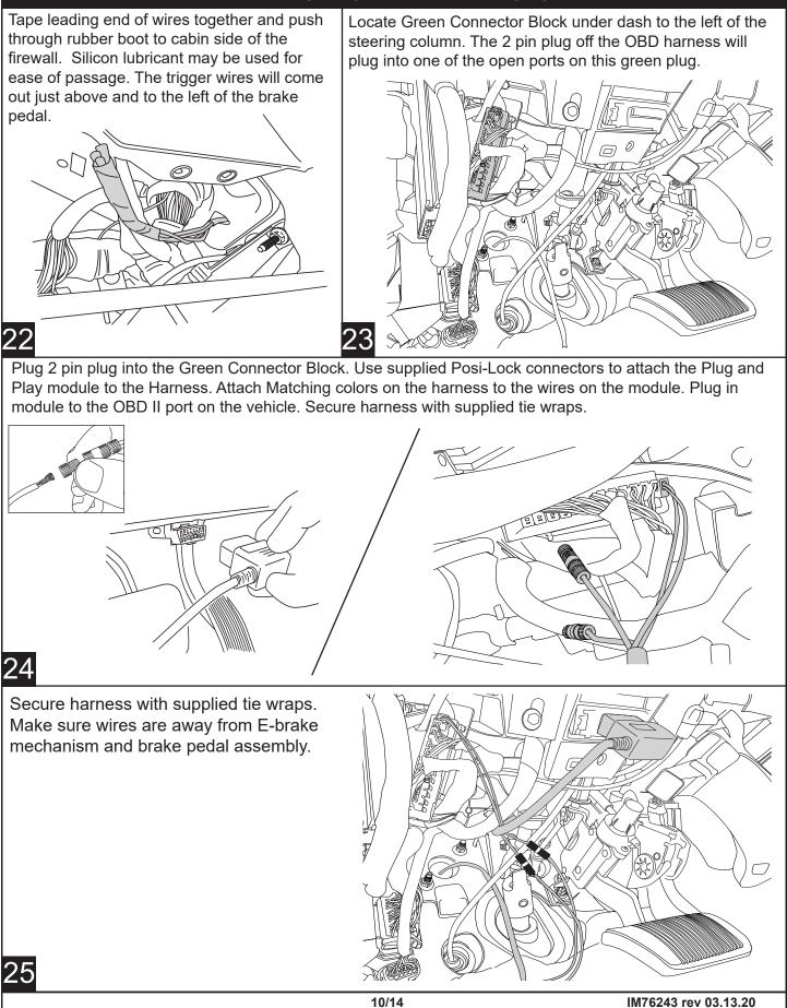
**OBD II install:** Use Supplied Posi-Lock connectors to attach the Plug and Play Module to the Harness. Attach matching colors on the harness to the wires on the module. Plug in module to OBD II port on the vehicle. Secure harness with supplied tie wraps. *Note: If the OBD II pass thru harness (76404-01A) was purchased see install sheet supplied in packaging. The*
