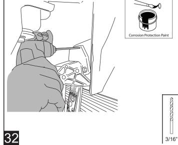
Using a Rivet Gun install rivets.
