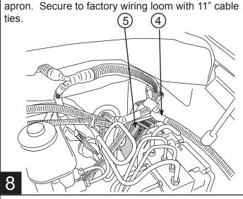
Install controller under hood on driver side fender
