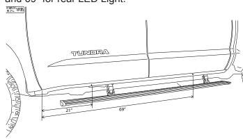
Drill a 9/32" hole through the pinch weld at marked locations. Deburr all holes.
