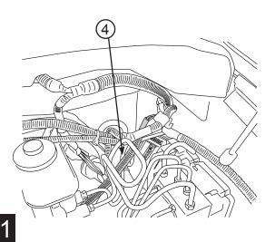
Insert plug from wire harness onto motor.
