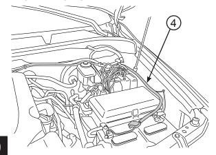
Route longest leg of wire harness across fire wall to passenger side and under vehicle outside of frame rail.
