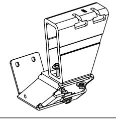
Assemble Linkage to bracket assembly using a 15mm Socket or wrench. Use supplied flange Bolts (#9). Torque Bolts to 20ft-lbs.
