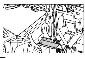
Offset step pad forward and secure using provided PT Screws. Tighten to 5ft-lbs using a T25 Torx bit. Verify Step pad alignment to body line of vehicle. Once step pad is in line to vehicle torque all bracket hardware to 16ft-lbs.
