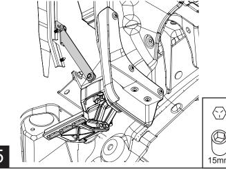
Using supplied M8 hardware Bolts(#12) Nuts (#13) and M10 bolt (#9) and nut (#8) mount frame support bracket to lateral bracket as shown.
